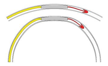
Figure 17. Schematic view of a pre-ferrulized cable with attached air-suction pig. Above the curvature that can be passed according to equation 1. Below a much sharper bend is passed when the air suction pig pulls the pre-ferrulized cable through the bent microduct while deforming it locally
