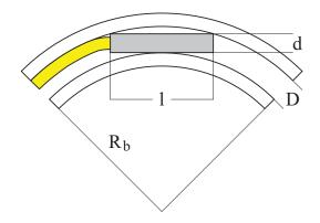
Figure 4. Schematic view of a preferrulized cable in a section of bent microduct
