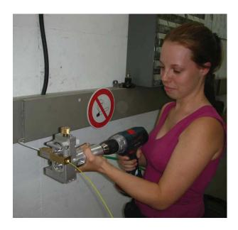
Figure 9. New pushing machine for battery-powered drilling machine, with clip-on inserts like blowing heads. The latter is mounted on this picture
