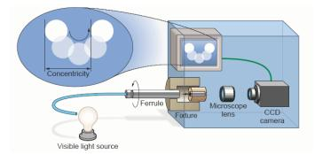
Figure 2. Schematic view of active core alignment
