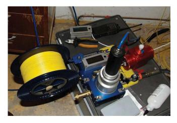
Figure 12. Blowing from a small spool
